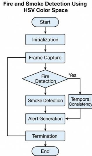
Figure 1: Process Flowchart
